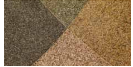
Translucent tints give add color without hiding the underlying concrete
